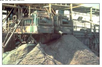
Figure 1. Shale Shaker on an Oil Rig
